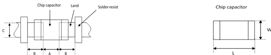
Recommended land dimensions for reflow-soldering
